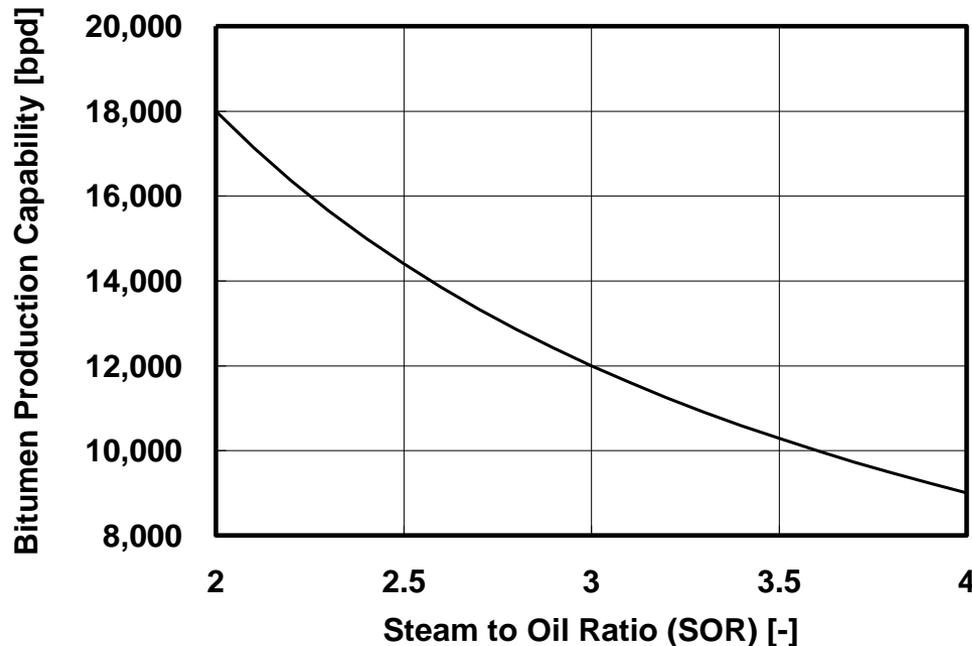
✓ One unit of 4S-135 MWt supplies steam for a relatively small SAGD plant to produce approx. 12,000 bpd of bitumen (@ SOR=3)
